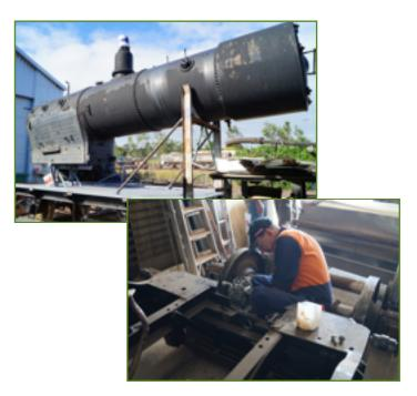
All work on C16-106 is working towards reuniting the mainframe with the driving wheels and lowering the main frames off the concrete blocks. The locomotive needs to be trammelled, this is when the driving wheels are set perpendicular to the connecting rod, set parallel to each other and set at the exact coupling rod spacing. This is a critical and important stage, because if not done correctly the axle-boxes, coupling and connecting rod bushes will run hot and wear excessively.
